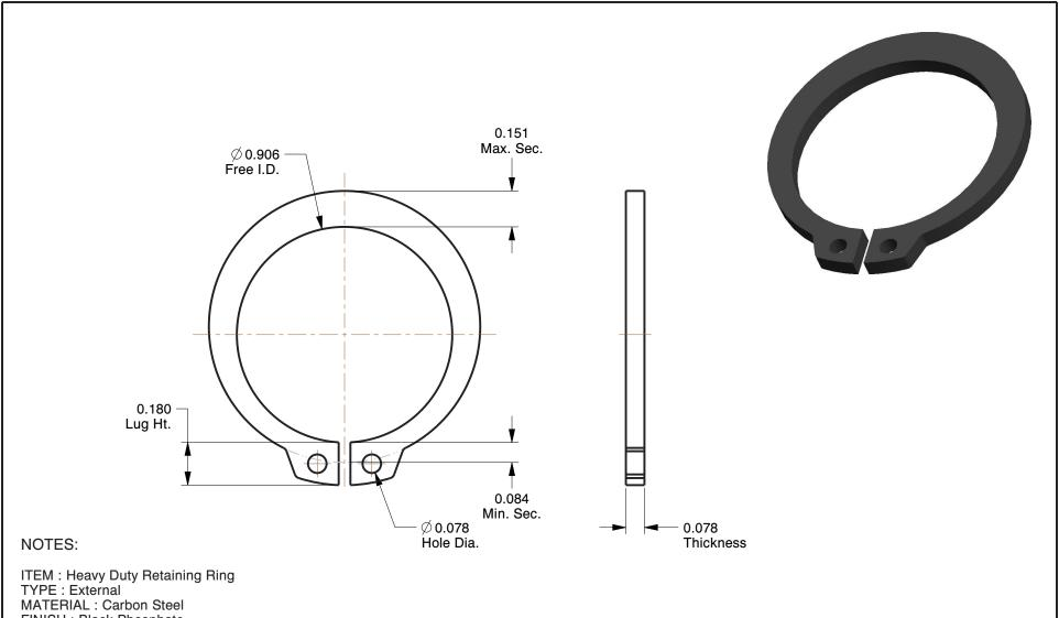
MATERIAL: Carbon Steel FINISH: Black Phosphate FOR SHAFT DIA: 1" PACKAGE QUANTITY: 10
