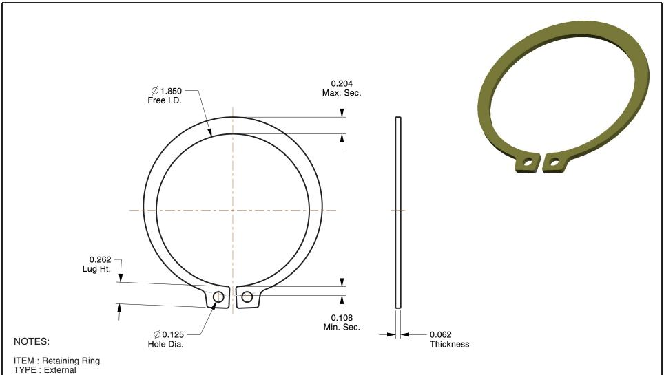
MATERIAL: Carbon Steel FINISH: Yellow Zinc FOR SHAFT DIA: 2" PACKAGE QUANTITY: 10
