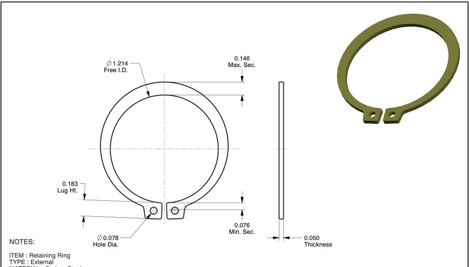
MATERIAL: Carbon Steel FINISH: Yellow Zinc FOR SHAFT DIA: 1-5/16" PACKAGE QUANTITY: 25
