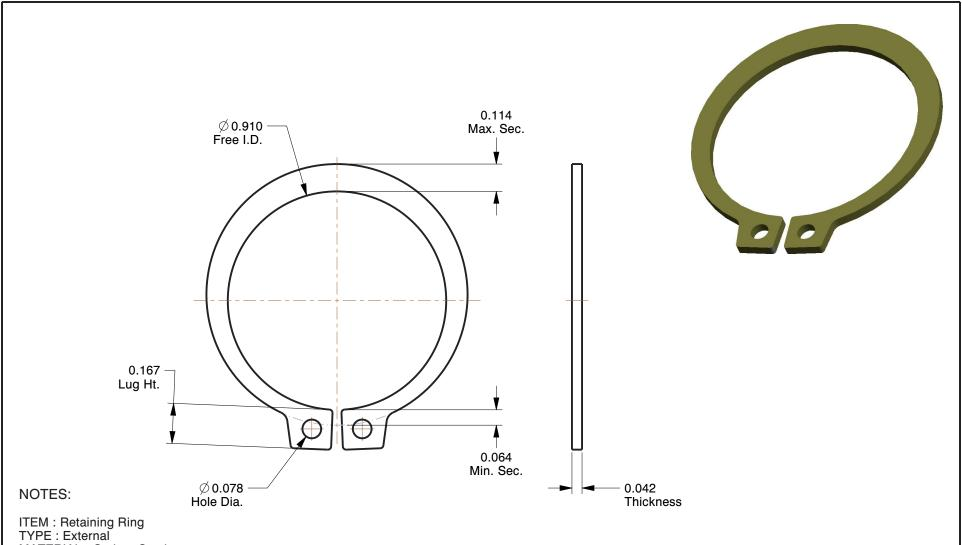
MATERIAL: Carbon Steel FINISH: Yellow Zinc FOR SHAFT DIA: 63/64" PACKAGE QUANTITY: 50
