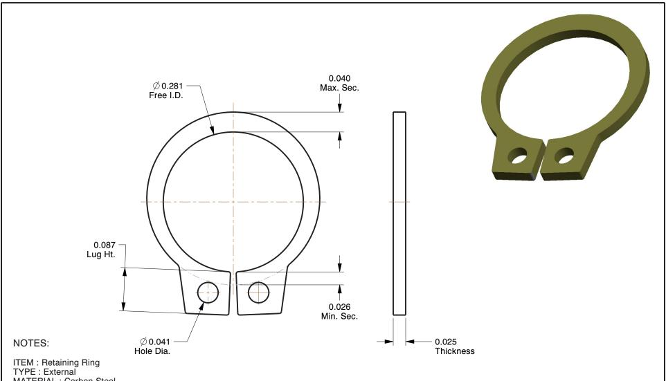
MATERIAL: Carbon Steel FINISH: Yellow Zinc FOR SHAFT DIA: 5/16" PACKAGE QUANTITY: 100
