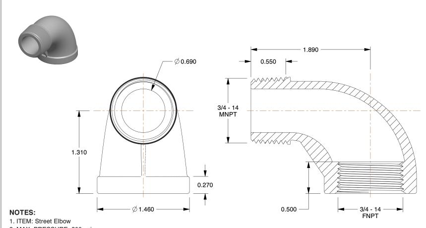
2. MAX. PRESSURE: 300 psi3. PIPE SIZE - PIPE FITTING: 3/4"
