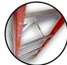
Full set of rear horizontals spaced one per foot
