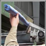
Our heaviest absorbent sock forms a barrier to prevent spills from spreading.
