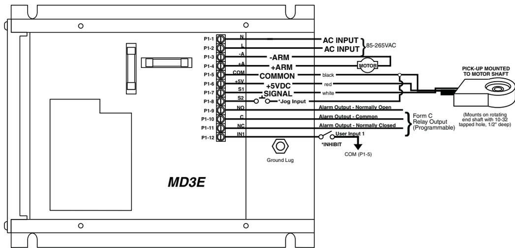
\* P1-8 & P1-12 user input may be programmed for a number of functions. Including (jog, inhibit, etc.)
