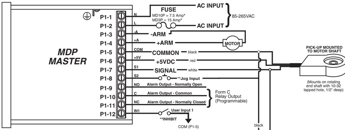
\* For AC inputs utilizing two hot lines, both inputs should be protected with appropriately sized fuses or circuit breakers.
