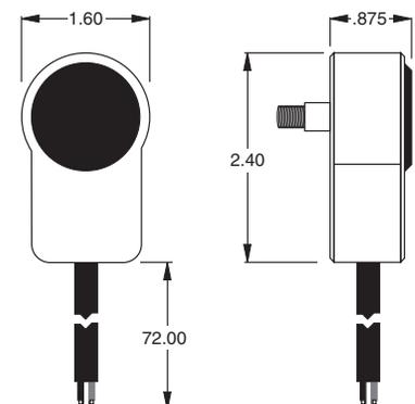
No other mounting screws are necessary, as the cord will keep the unit from rotating.
