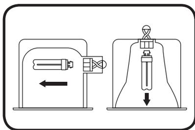
2 Remove the existing fluorescent lamps from the fixture and dispose of them properly based on local regulations.
