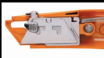
**Insert Blade** underneath blade retainer, aligning blade notch with alignment tab. Close cutter body, rotating wheel clockwise to tighten. Dispose of used blade safely.
