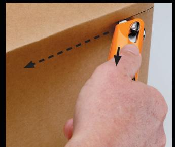
**Release thumb pressure and place thumb on cutter body** and continue the cut. Friction will maintain blade exposure. Blade will automatically retract at the end of the cut.
