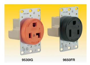
Three-wire configurations feature single side pressure screw terminal design allowing top access to all three terminals for easy wiring. NEMA line numbers and ratings are molded into the face for easy identification. Isolated ground versions provide protection for sensitive electronic equipment by helping to limit electrical noise on the equipment grounding circuit.
