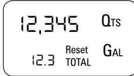
A few seconds after dispensing has ended, on the lower register, the display switches from Reset Total to General Total: the word RESET above the word TOTAL disappears, and the Reset Total is replaced by the General Total.
