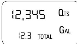
This situation, where only “TOTAL” is displayed, is called **STANDBY mode**. It remains stable until the user operates the meter again.
