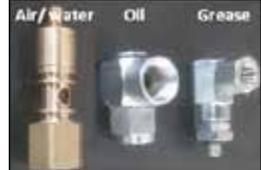
Inlet Swivel used in different Hose reels
