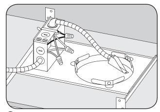
Connect conduit fitting to the existing junction box. Connect the black, white and green yellow wires of the input leads to the black, white and green AC line wires using UL Listed twist-on wire connectors and close the junction box.
