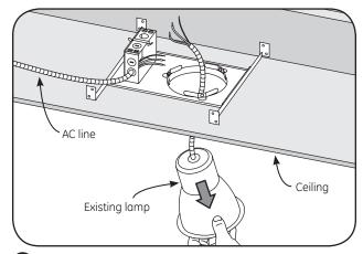
Remove existing lamps, ballast and reflector. Leave wiring in junction box. Verify that the AC supply line is provided with a ground wire connected to the luminaire.
