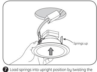
Load springs into upright position by twisting the springs upward and carefully insert the fixture to the hole of the frame. Ensure fixture is secure.
