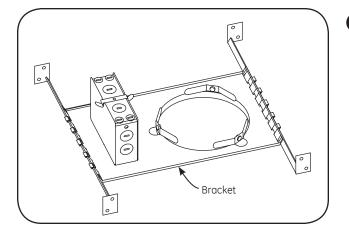
Before retrofit, verify that the junction box and bracket in the existing installation are metal and are constructed similarly to the illustration at left.
