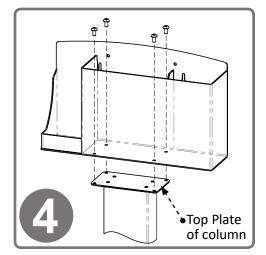
Attach the RS001-0512 Respiratory Hygiene Station to the column using (4x) screws included with stand. Tighten.
