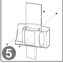
To mount the MP-070 Sign Holder, sandwich the holder over the top edge of the dispenser, lining up holes. With a flathead screwdriver, attach using (2x) barrel screws included with sign holder.
