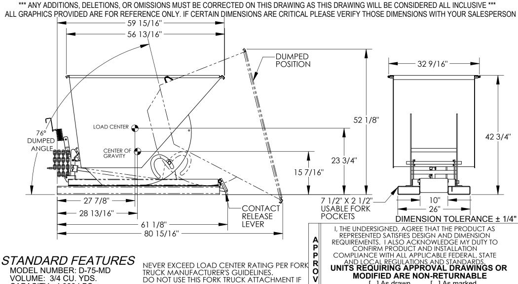
CAPACITY: 4,000 LBS. OVERALL WIDTH: 32 9/16" **OVERALL LENGTH: 61 1/8"** OVERALL HEIGHT: 42 3/4" PULL CABLE IS AT LEAST: 48" TOUGH BAKED IN POWDER COATED BLUE FINISH
