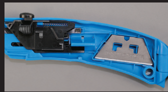
Remove spare blade from blade compartment. Use only S Series replacement blades: #SP-017, SPD-017 or PBDSP017B.
