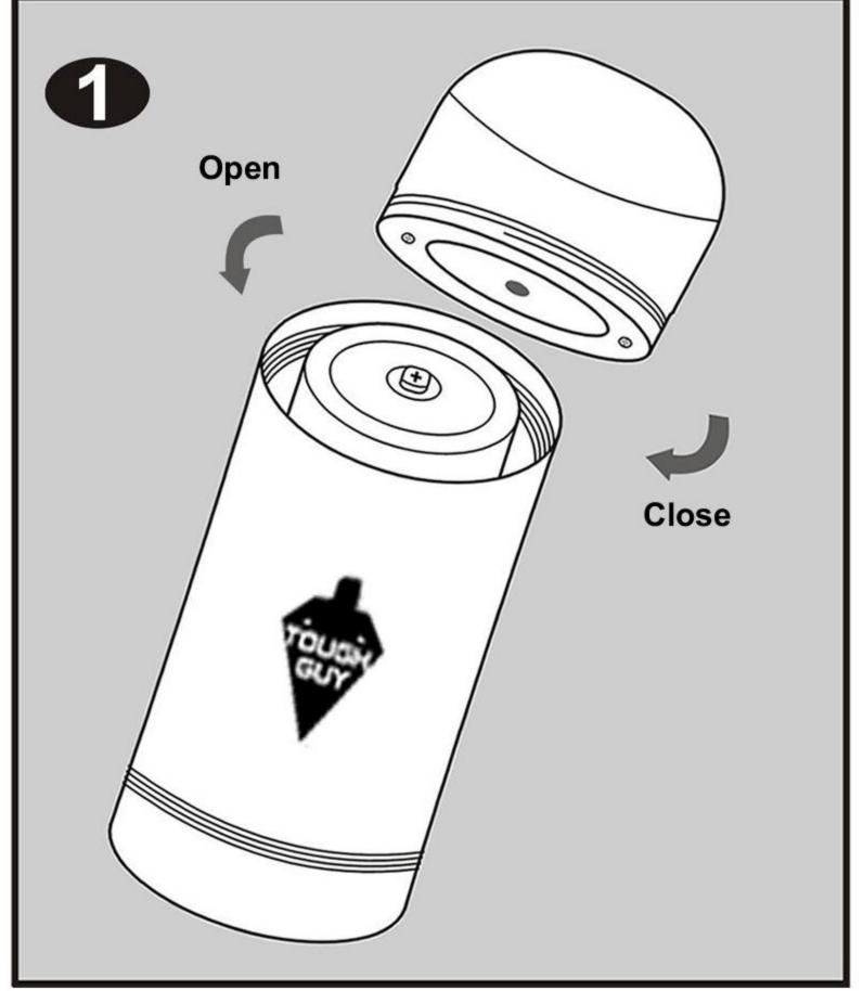
Turn the lens head counter-clockwise to remove it from the battery case. Turn the lens head fully clockwise to secure it in place.
