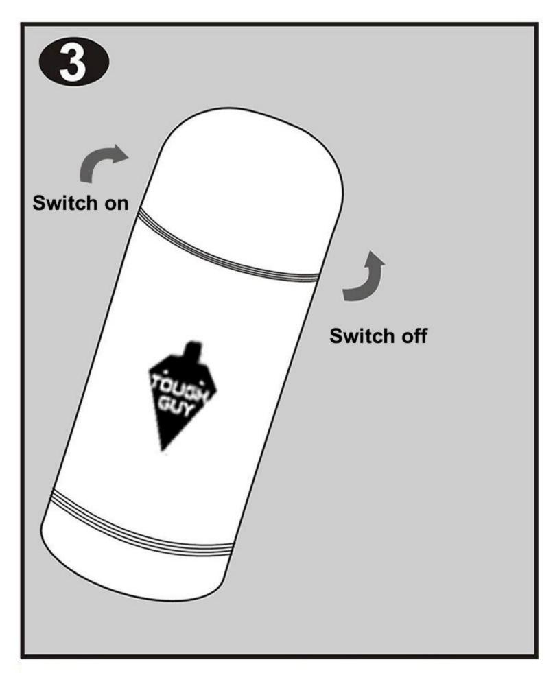
Turn the lens head fully clockwise to activate the flashing light. Turn the lens head approximately 1/4 turn counter-clockwise to de-activate the flashing light.
