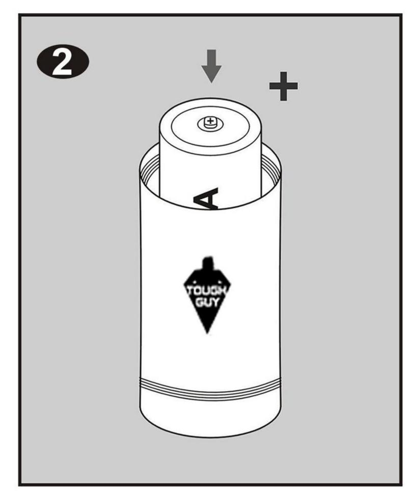
Insert one D size battery into the battery case as shown in the diagram.
