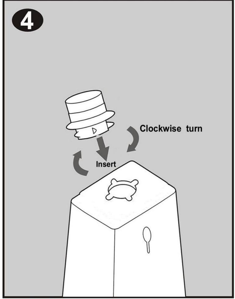
Insert the adapter into the top hole of the cone and turn it approximately 1/4 turn clockwise to lock it into position.
