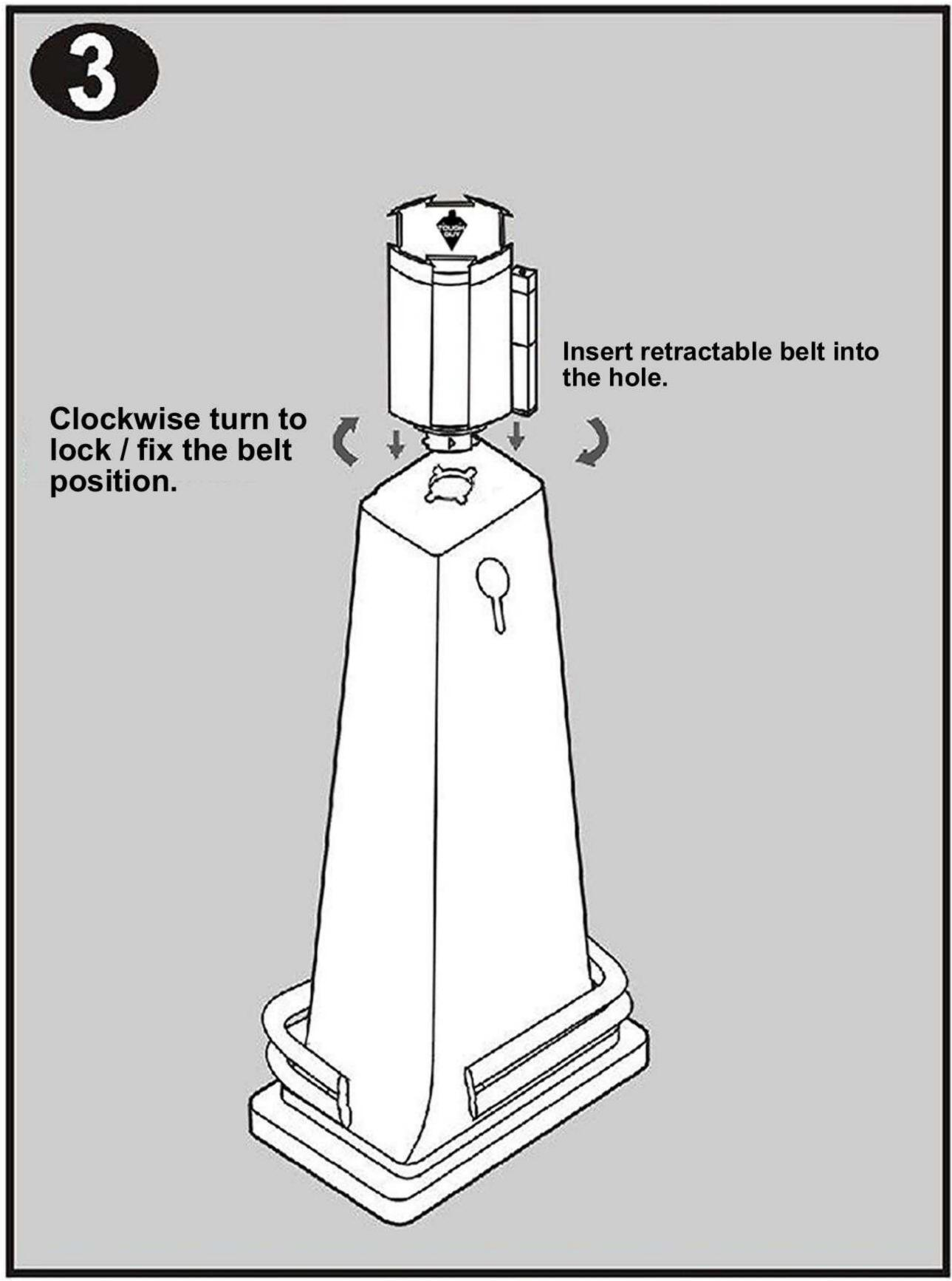
Insert the retractable belt assembly into the top hole of the cone and turn it approximately 1/4 turn clockwise to lock it in place.
