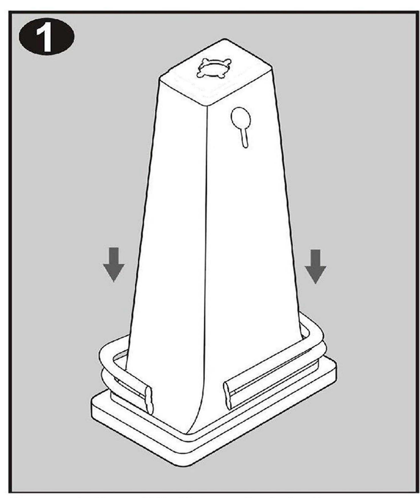
Insert the 20 lb.weight ring from the top of the cone to the bottom of the cone slowly and gently.
