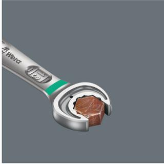
The Joker's clever double-hex geometry delivers a very positive connection with nuts or bolts – it's a perfect fit. And the exchangeable, hardened metal gripping plate in the Joker's mouth literally bites itself into the bolt, with its extremely hard tips. Both features combine to prevent slipping, even at higher torque.
