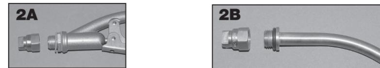
Attach nozzle to shut-off handle or extension wand.
