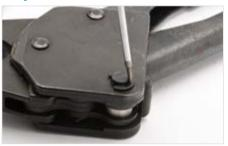
Remove existing E-Clip by prying it away from the pin with a flat head screw driver (or needle nose pliers).
