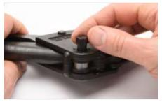
2. Lay the tool flat with the adjustment numbers facing up. Insert the spacer and align the path for the pin with the screwdriver. Push the pin through the hole making sure the pointer on the pin is aligned with the appropriate number on the tool. Moving the tools handle back and forth while pushing the pin helps to seat the pin.
